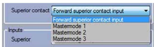
For information about setting this up, see the section "Serial connection of several iVent 8A ventilation control panels". When supplied the mode is pre-set to "Forward superior contact input".
